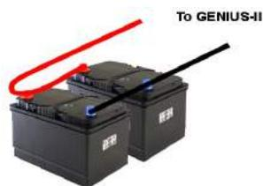
Figure 4: Recommended wiring for connecting batteries in parallel
